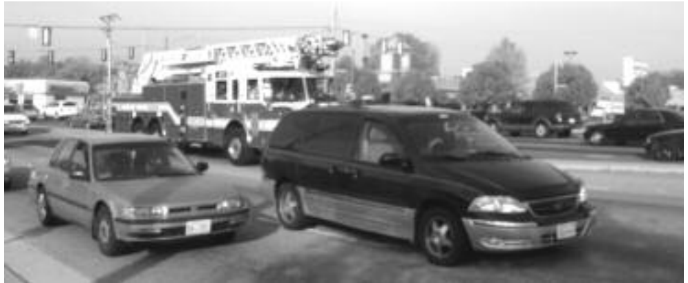
Figure 9 – A Ladder Truck Without EVP Pushes Through a Queue at a Red Signal
